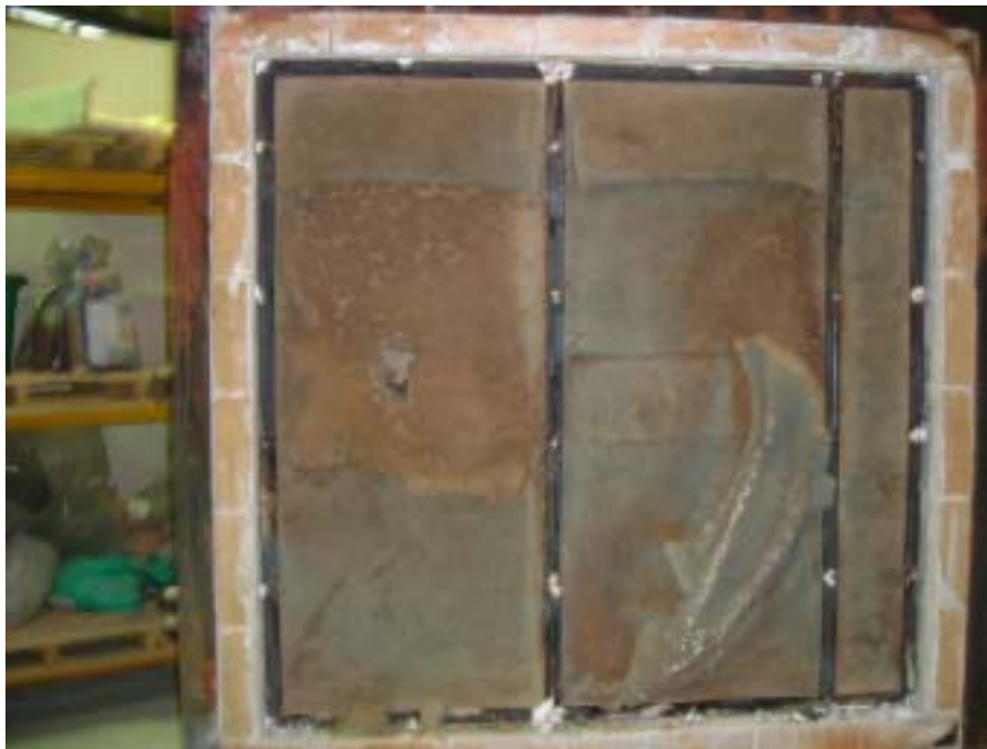
Figure 8 – Post Test of Fire Side Test Panel 1
