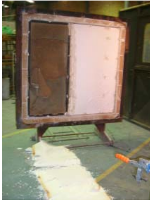
Figure 7 – Post Test of Fire Side of Test Panel 1
