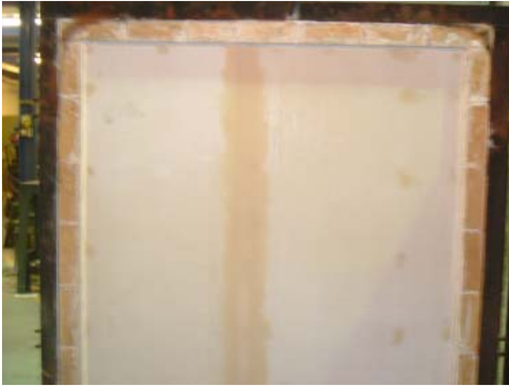
Figure 3 – Pre Test View : Fire Side Test Panel 1
